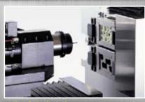
The CAM system is also one of the most flexible on the market, manufacturing restorations from a wide variety of materials including composites bonded titanium, Vita InCeram Alumina and Zirconia all-ceramic, and the extremely strong Zirkon (zirconium oxide).
